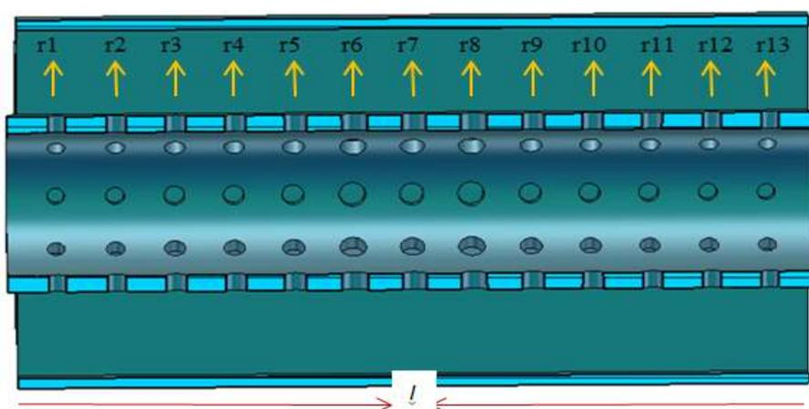
Figure 4. Cross-sectional view of mode coupler
