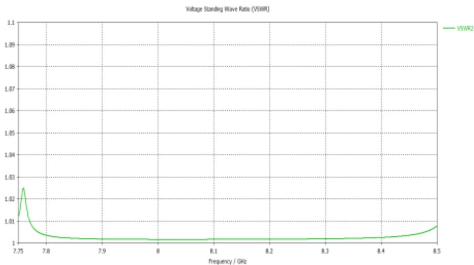
**Figure 10. Simulated VSWR at input Port 2**
