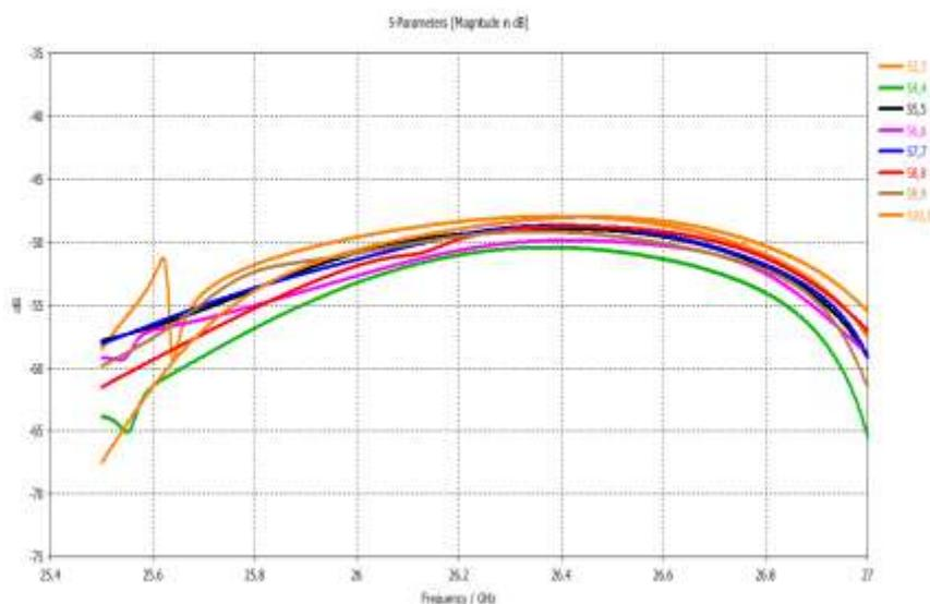
**Figure 7. Return loss characteristic of sum ports at 25.5-27GHz**
