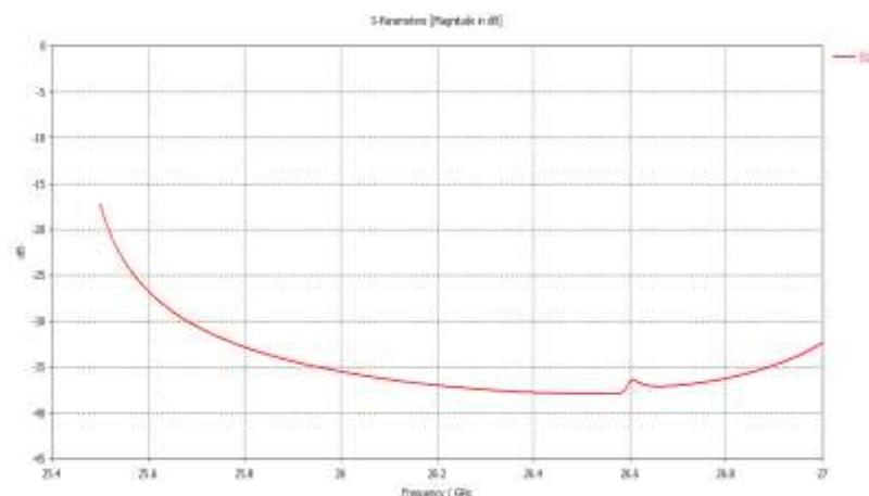
**Figure 5. Input Port return loss characteristic at 25.5-27GHz**
