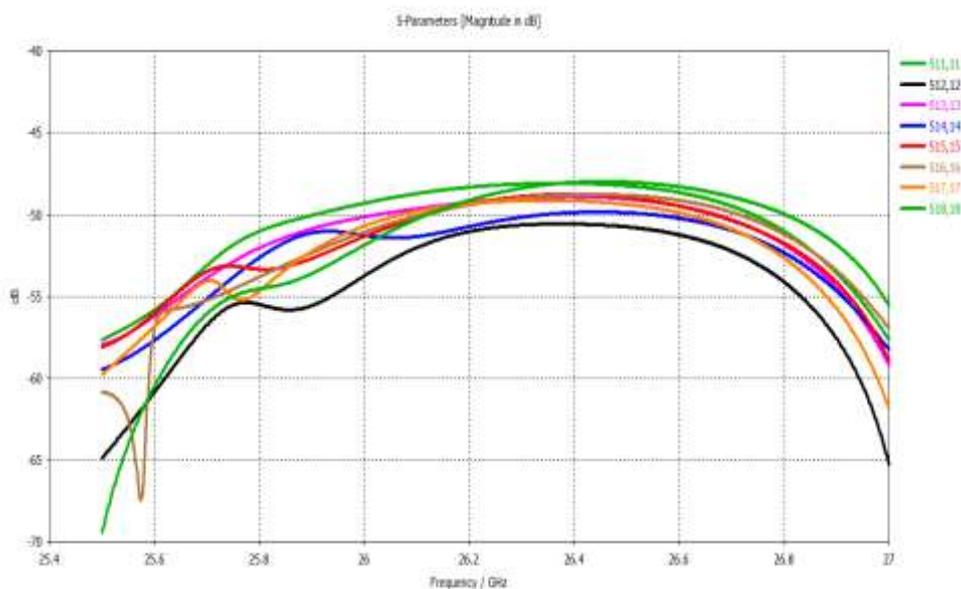
**Figure 8. Return loss characteristic of difference ports at 25.5-27GHz**
