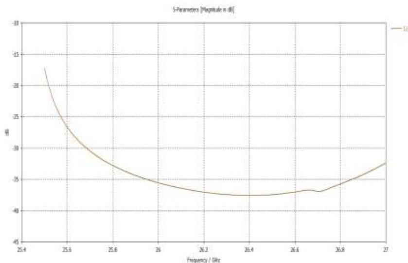
**Figure 6. Output Port return loss characteristic at 25.5-27GHz**
