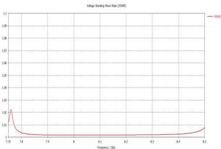
**Figure 9. Simulated VSWR at input Port 1**
