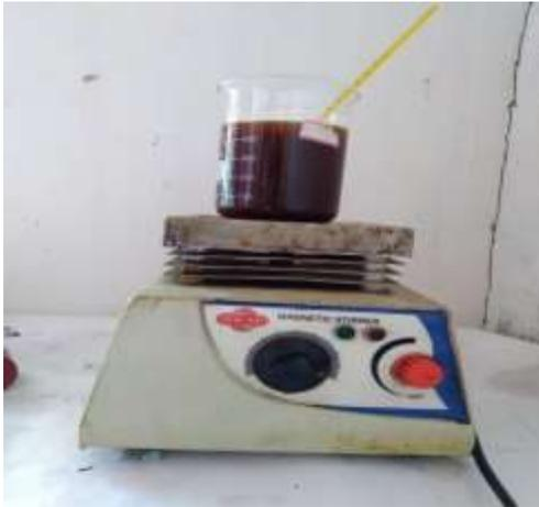
**Fig. 1 Heating of Oil to remove Water Particles**
