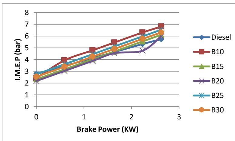
**Fig 9: Brake Power Vs Indicated Mean Effective Pressure**
