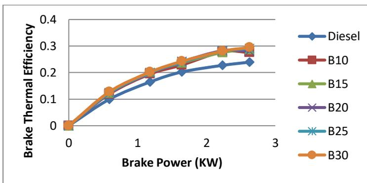
Fig 5: Brake Power Vs Brake Thermal Efficiency
