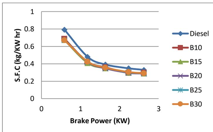
**Fig 7: Brake Power Vs Specific Fuel Consumption**
