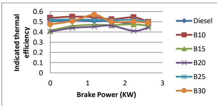
Fig 6: Brake Power Vs Indicated Thermal Efficiency
