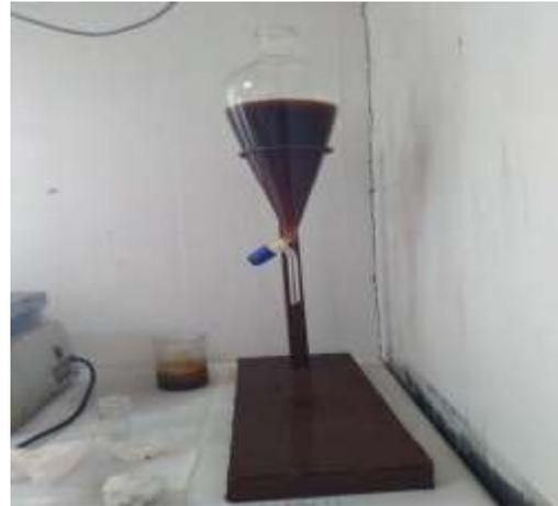
**Fig. 2 Sedimentation of Glycerol and Biodiesel**
