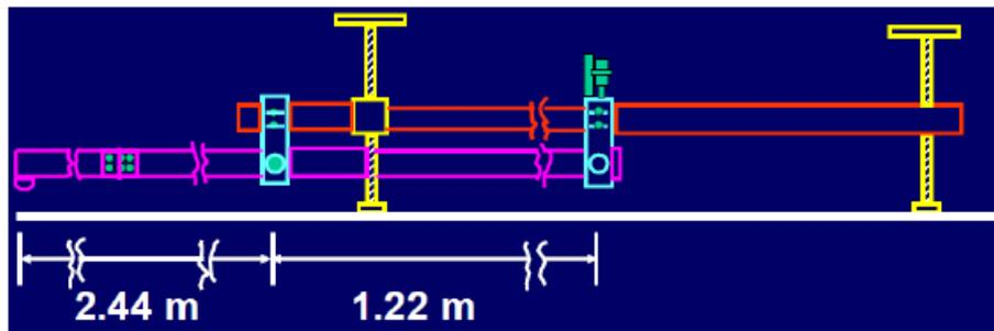
Figure 2: Cross-section of Benkelman Beam
