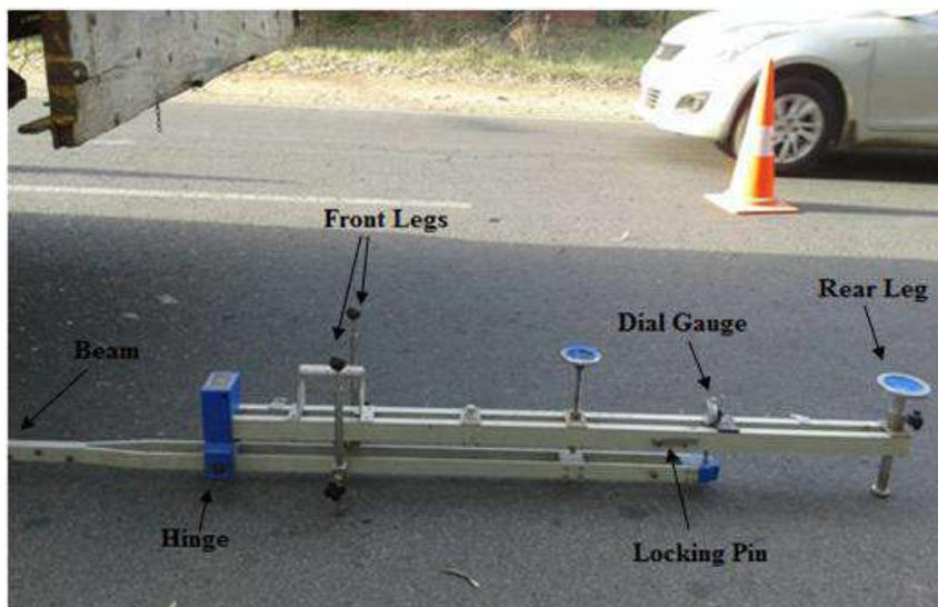
Figure 1: Benkelman Beam mounted on Rear-Axle
