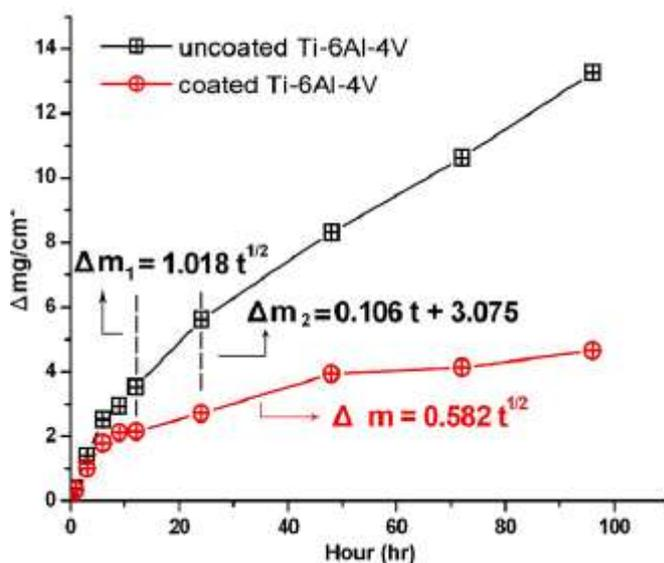
Fig.01; Weight change curves obtained for uncoated and coated Ti-6Al-4V specimens during oxidation at constant temperature of 800 °C in air. Shiang-Cheng [14]
