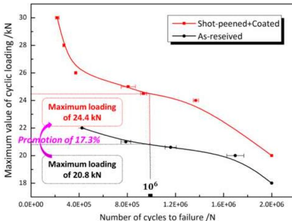
Fig (05); Fretting fatigue lives of the AS and SC specimens under different loading conditions (QI YANG <sup>[27]</sup>)
