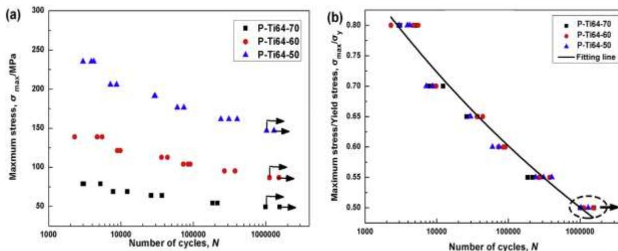
Fig (04); The  $S-N$  curves of porous alloys (Ti6Al4V) using absolute (a) and normalized (b) Stress values. The arrows represent porous samples that did not fail. Fuping Li<sup>[23]</sup>
