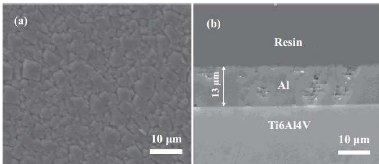
Fig (03); cross section morphology of magnetron sputtered Al layer on Ti6Al4V (Shi-hang Kang<sup>[21]</sup>)
