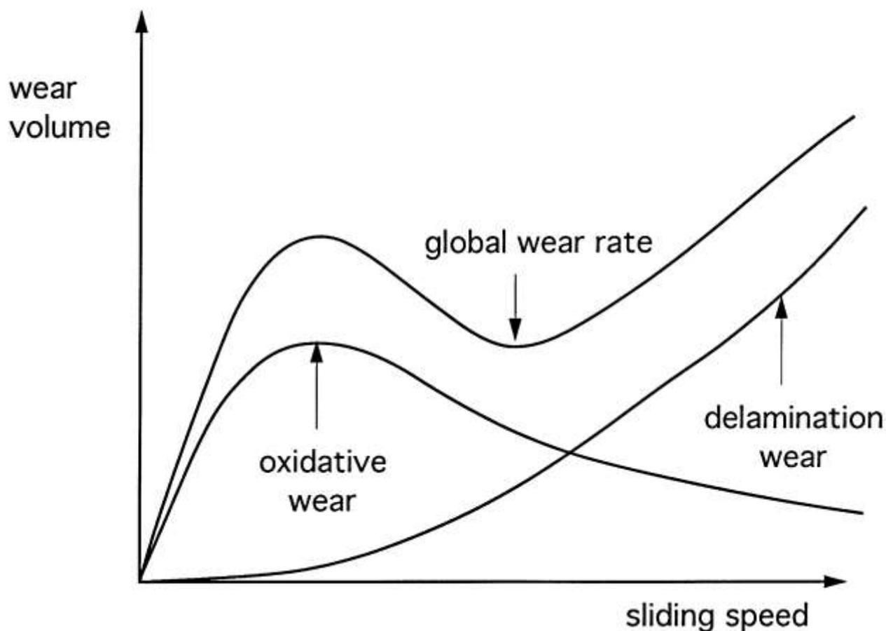
fig (02); The qualitative representation of sliding wear VS sliding speed (Molinari<sup>(17)</sup>)
