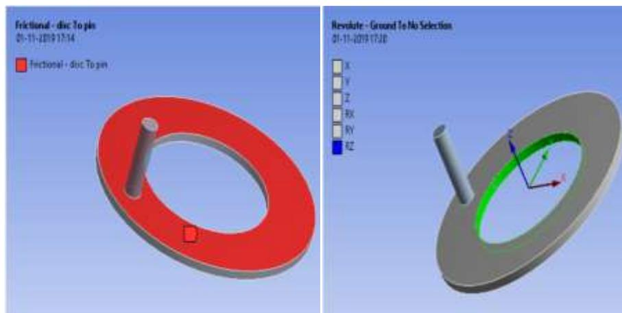
**Fig 1.3 the friction between the contacts & revolute joint**
