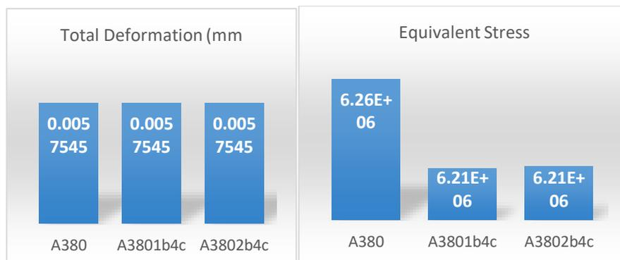
**Fig 1.7 Total Deformation & Von – Misses Stress of A380, A380+1%B4C & A380+2%B4C (90N)**
