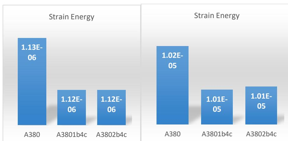
**Fig 1.8 Strain Energy of A380, A380+1%B4C & A380+2%B4C (30 & 90N)**
