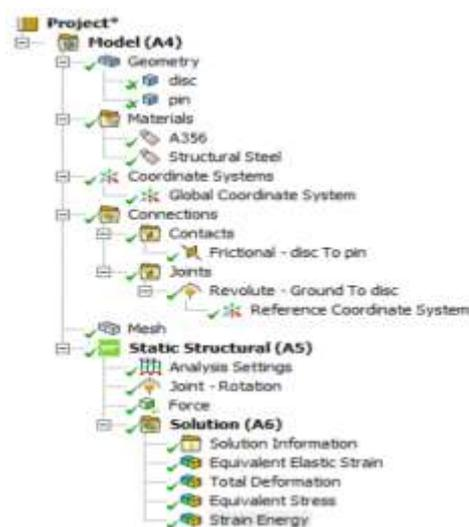
**Fig.1.2 The Detailed project structure of the pin on disk analysis**
