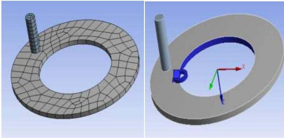
Fig 1.4 the meshing & revolution of the disc
