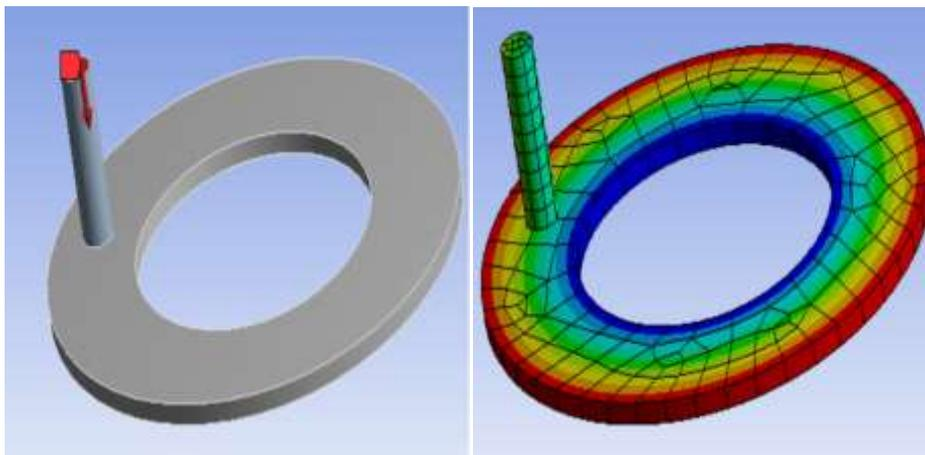
Fig 1.5 Force on pin in Z-direction & total Deformation on Pin – On- Disc (30N)
